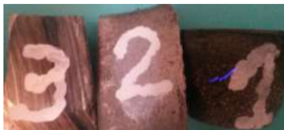
Figure 3. Samples of white wear-resistant cast irons. 1 - 280X29NL, 2 - 300X32N2M2TL, 3 - 330X17L
